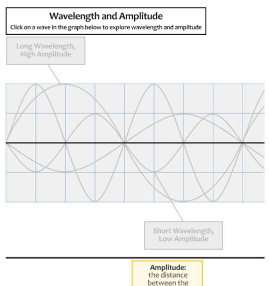
The waves from power lines and electrical devices have a much lower frequency than other types of EMR, such as microwaves, radio waves or gamma rays. However, a low frequency wave does not necessarily mean that it is low energy; a charging cable for a phone produces a low frequency, low energy electromagnetic field, while a high-tension power line can create a much higher energy
